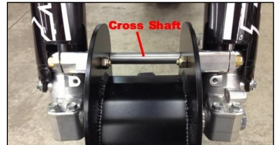
Install them onto the bike using only the two outside screws to hold them on. The inside screws will not be able to be reinstalled due to this portion being cut away.
